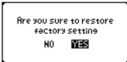
Hold the **PLAY** button for 2 seconds, rotate the **VALUE** control to switch “Yes” or “No” to restore factory setting.
