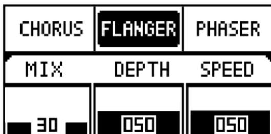
Press the **MOD** button to access the Modulation effect page. Rotating the **VALUE** control knob will select different types of Modulation effects. Pressing the **VALUE** control will select the various parameters which can then be adjusted by rotating the **VALUE** control knob. Pressing the **MOD** button at any time while on this page will return the parameter selection back to the modulation type selector.
