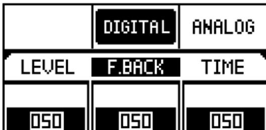
Press the **DLY** button to access the Delay effects page. Rotating the **VALUE** control knob will select different types of Delay effects. Pressing the **VALUE** control will select the various parameters which can then be adjusted by rotating the **VALUE** control knob. Pressing the **DLY** button at any time while on this page will return the parameter selection back to the delay type selector.
