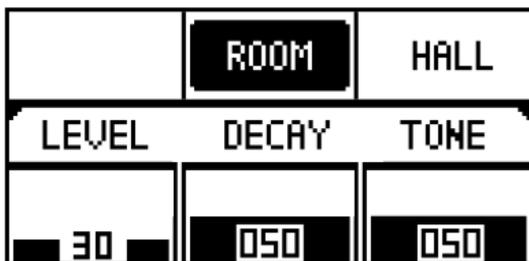
Press the **REV** button to access the Reverb effects page. Rotating the **VALUE** control knob will select different types of Reverb effects. Pressing the **VALUE** control will select the various parameters which can then be adjusted by rotating the **VALUE** control knob. Pressing the **REV** button at any time while on this page will return the parameter selection back to the Reverb type selector.
