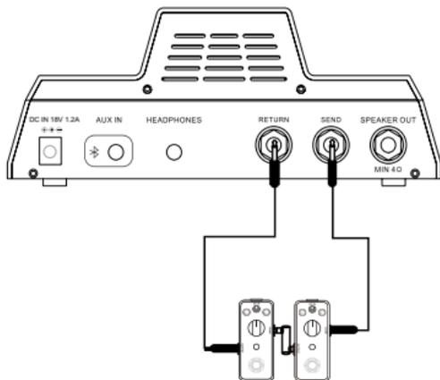
Connect the **SEND** from the D15 to the input of your external effects. Connect the output of your external effects to the **RETURN** of the D15.
