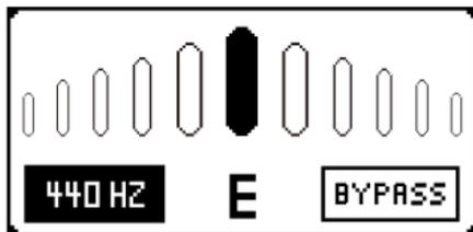
Press the **TUNER** button to access the tuning function page. The tuner is set to A=440Hz as stock, rotate the **VALUE** control to change this calibration.
