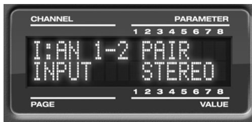
Figure 4-5: The settings for analog inputs 1 and 2 (as a pair).
