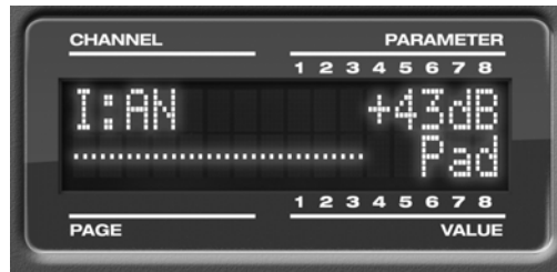
Figure 6-2: the LCD provides feedback when you adjust the Precision Digital Trim and pad for the four mic/guitar inputs.
