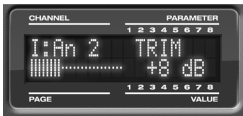
Figure 4-6: Setting the input trim for a TRS analog input.
